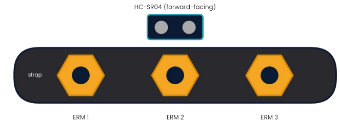
Top view: forward-facing sensor and three honeycomb-arranged motors.
